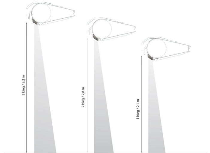
PIC. 2.2 AIR STREAM RANGE FOR DIFFERENT FAN STEPS
